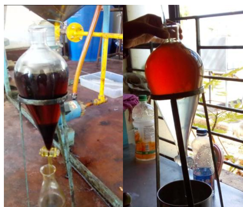
Fig.6 Washing of biodiesel.
